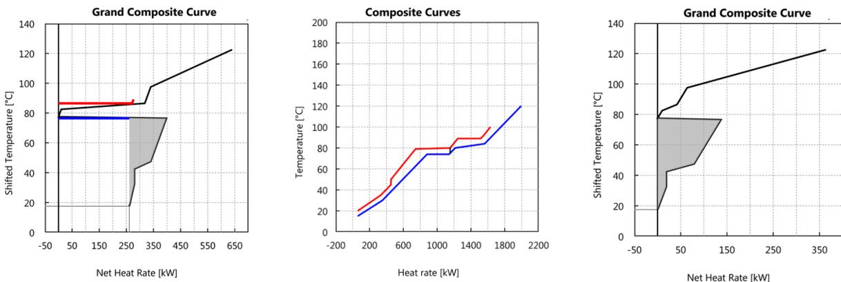
**Figure 10: Heat pump matched against GCC (left), CCs after heat pump streams integration, but not yet deciding evaporator and condenser heat transfer matches (center), and GCC after taking out actual evaporator and condenser heat transfer matches (right) – Scenario 1 involving a 276 kW compression heat pump.**
