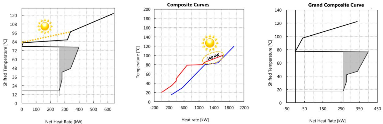
**Figure 11: Solar heat integration ( $340 \text{ kW}$ ) matched against GCC (left), CCs after  $340 \text{ kW}$  solar heat integration (center), and GCC after taking out  $300 \text{ kW}$  solar heat supply actually matched with lye bath (right) – Scenario 3 solar heat supply.**
